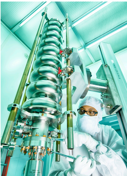
These “superconducting” niobium cavities, constructed at Fermi National Accelerator Laboratory, allow radio frequency fields to boost electron energies practically without electrical resistance. (R. Hahn/Fermilab) Top: An electron beam travels through a niobium cavity. (Greg Stewart/SLAC National Accelerator Laboratory)
