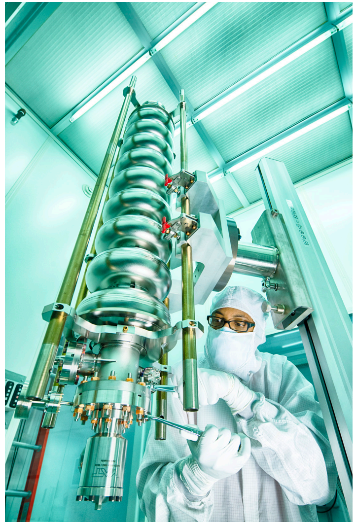
Cooled to minus 456 degrees Fahrenheit, these niobium cavities allow radiofrequency fields to boost electron energies without electrical resistance. Cryomodules—consisting of eight niobium cavities each—are a key component of LCLS-II's superconducting linear accelerator. (R. Hahn/Fermilab)
